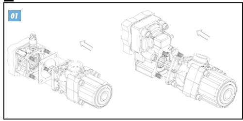
Fit the pump onto the PTO placing the gasket included in the mounting kit
