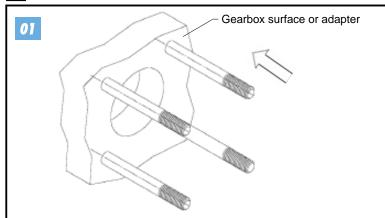
Using Loctite (medium sealing – Loctite 243, Loxeal 55-03 or similar), install the studs supplied with the mounting kit with a 30Nm tightening torque.
