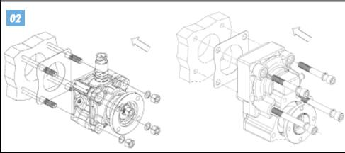
Place mounting gaskets included in the mounting kit and fit the PTO onto the gearbox. Screw the nuts with driving torque 80 Nm
