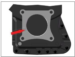
1) Take out the original rear cover and remove any presence of sealant or painting.
