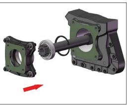
2) Fit in the gearbox the complete quill shaft.
